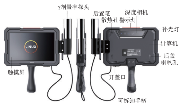
图 1 \gamma 剂量率辐射场测绘装置结构 Fig. 1 Structure of \gamma dose rate radiation field mapping device
