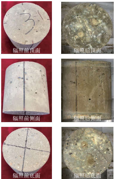
图 7 混凝土标准试样辐照前后的外形 Fig. 7 Outline diagram of standard concrete sample before and after irradiation
