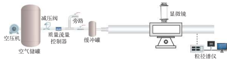
图 2 连续再悬浮实验平台示意图 Fig. 2 Schematic diagram of continuous resuspension experimental platform
