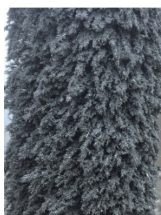
图 6 电解精炼所得金属铀枝晶产品 Fig. 6 Dendritic metallic uranium product obtained by electrorefining
