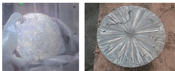
图 7 高温蒸馏纯化所得金属铀锭(a)及回收的镉锭(b) Fig. 7 Metallic uranium ingot (a) and cadmium ingot (b) obtained by high-temperature distillation purification
