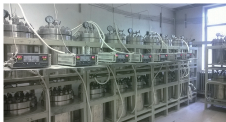
图 12 玻璃固化体多重屏障条件处置行为研究实验装置 Fig. 12 Experimental apparatus for research of disposal behavior of simulated glass wasteform under multi-barrier system conditions
